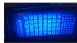
IDEXX Enterolert Quanti-Tray 2000, showing a positive (fluorescence) for enterococcus
