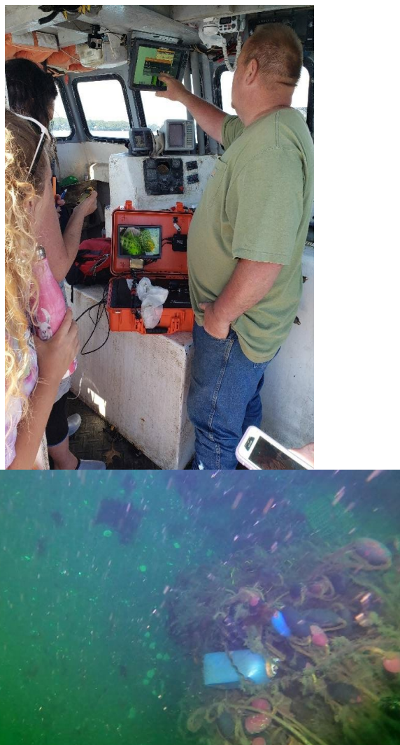
Figure 2. CFRF and Captain of F/V Nomad Casco Bay, Maine testing underwater video technology with sonar sighting of ghost gear (top) and image of ghost gear from survey (bottom).
