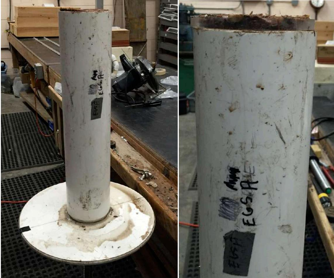
Figure 3: Spinning core extraction wheel and close up of 1 cm interval ready to be sliced off core.
