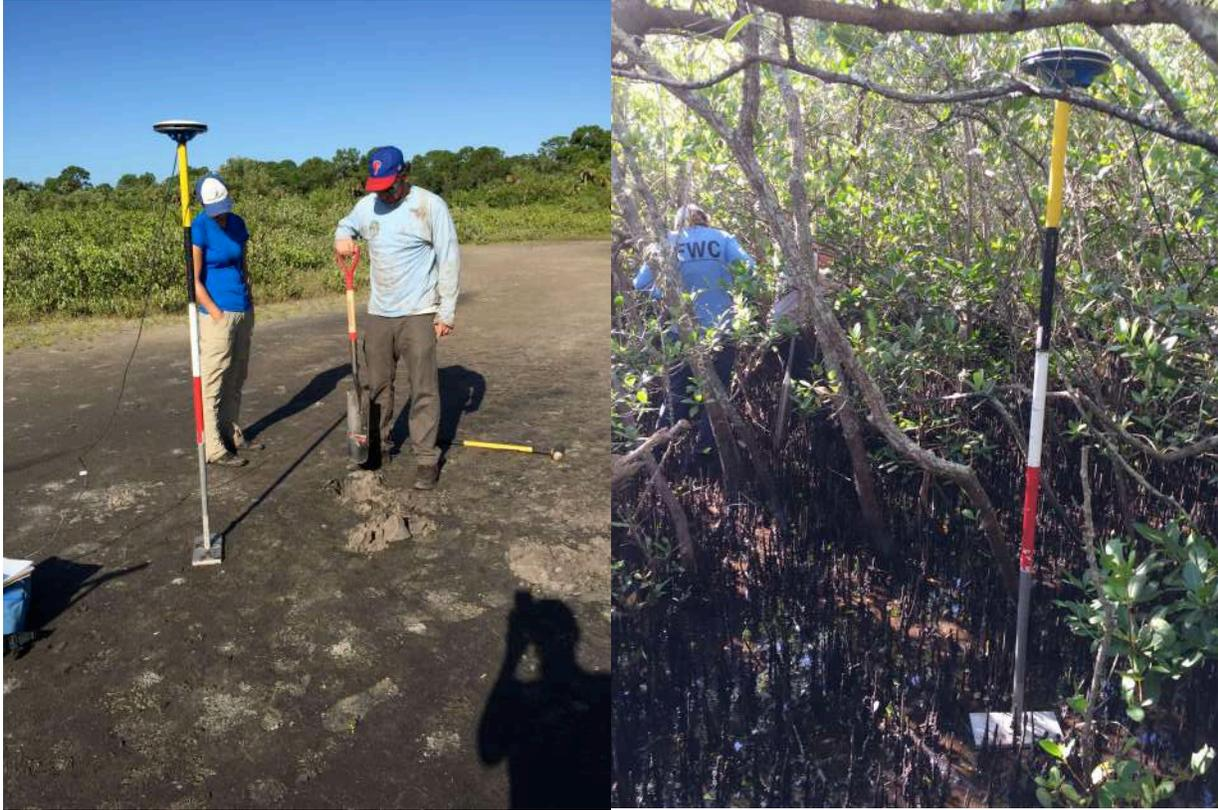
Figure 2: Differential GPS antenna at Upper Tampa Bay salt barren site and E.G. Simmons mangrove site. Antenna is clearly below the canopy at the mangrove site.
