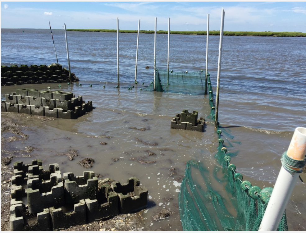
Block net surrounding newly constructed structured habitats in Nantuxent Creek at low tide. Image credit: Kurt Cheng, PDE
