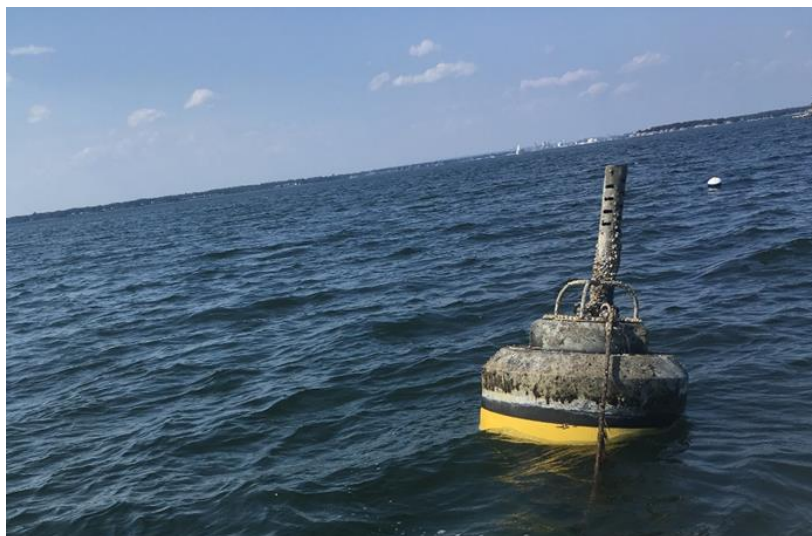
Figure 6. During the late summer of 2020, the buoy system counterweight was damaged on the Conimicut Pt Buoy causing the station to flip. Staff were able to get out to the site quickly and no real damage was done to the station. A new counterweight was installed and the station operational again in a few days.
