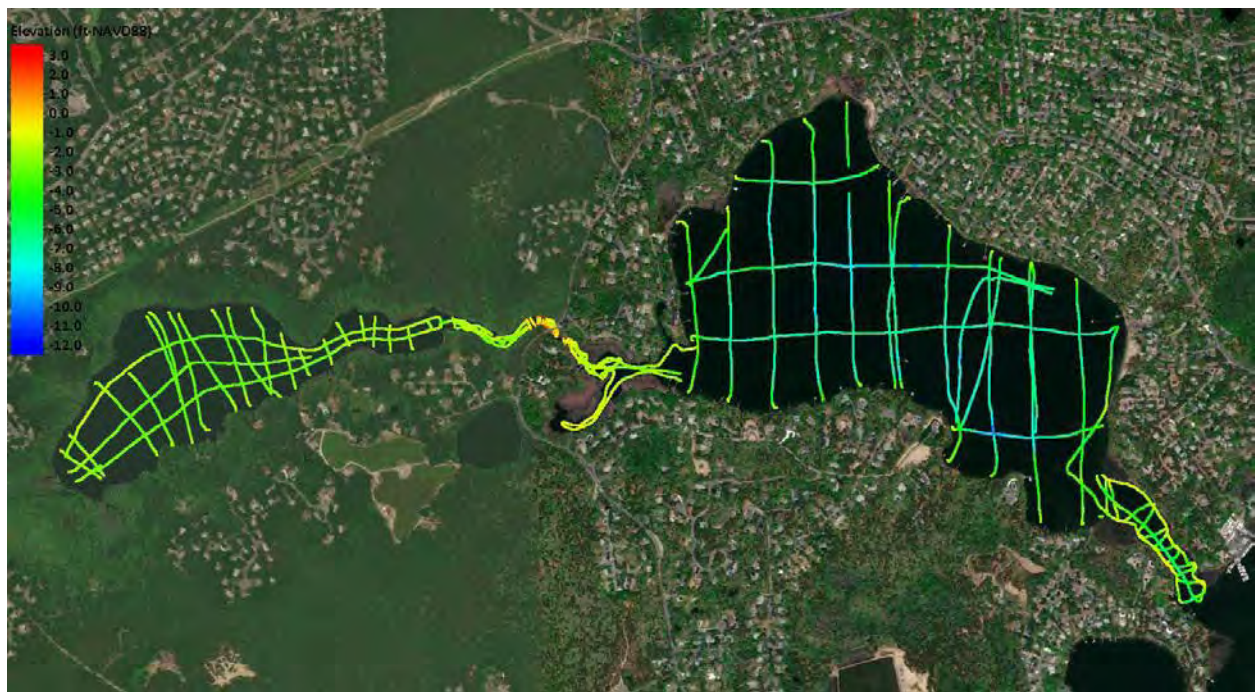
Figure 8. Hydrographic survey conducted on October 1, 2020.
