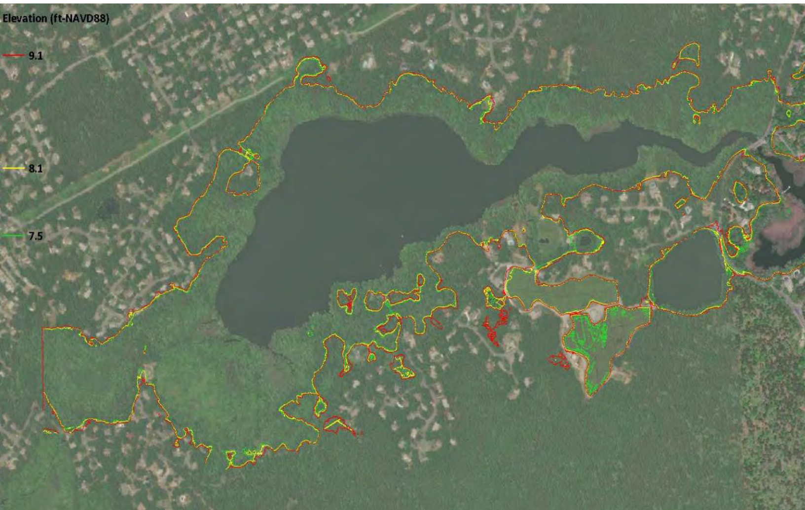
Figure 32. Contours of the 1% Annual Exceedance Probability (AEP) storm event. Red shows the FEMA flood elevation, yellow shows the modeled peak elevation with seiche, and the green line is the elevation from the Massachusetts Coastal Flood Risk Model (MCFRM).
