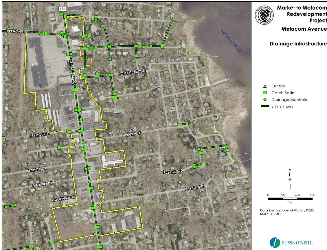
Figure 14. Metacom Avenue Drainage Utilities/Infrastructure
