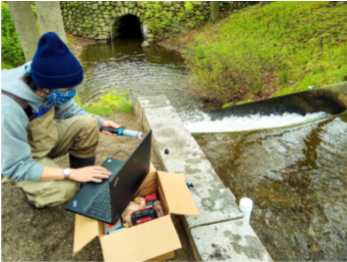
Will Helt of the Nature Conservancy installing a pressure transducer to measure water level at the outflow of RWP.
