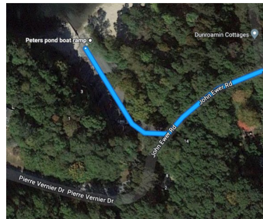
Figure 9: Aerial view of the Peters Pond Boat Ramp showing the two private roads that are currently contributing to the drainage area due to malfunctioning catch basins. (Image from Google Earth)
